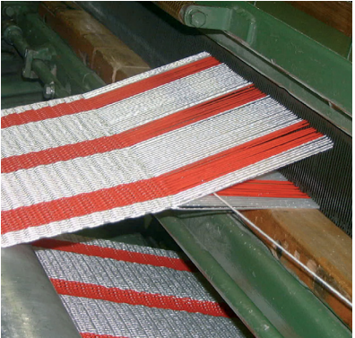
Ammeraal Beltech's in-house weaving and coating capabilities make it possible to offer a wide range of endless and non-endless fabric constructions, using natural (e.g. cotton, flax) and synthetic yarns (e.g. polyester, polyamide, aramid).
