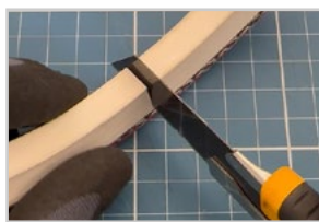
Cut the V-guide down to the mesh
