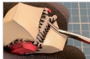
Pry up the pin using a pick
