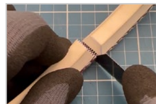
Carefully cut the coating of the belt
